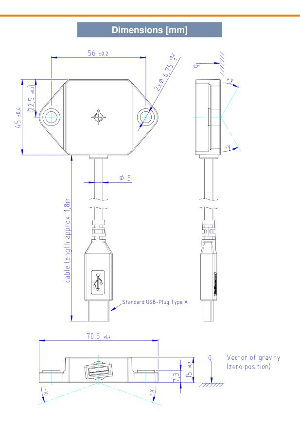
TE SENSORS /// AXISENSE-1 SERIES USB Tilt Sensor
