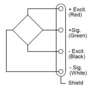
Note: for EPB-B0 thermal compensation is made with an external module
